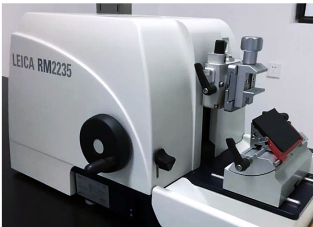
Figure 6. Leica RM2235 manually controlled rotary microtome.
