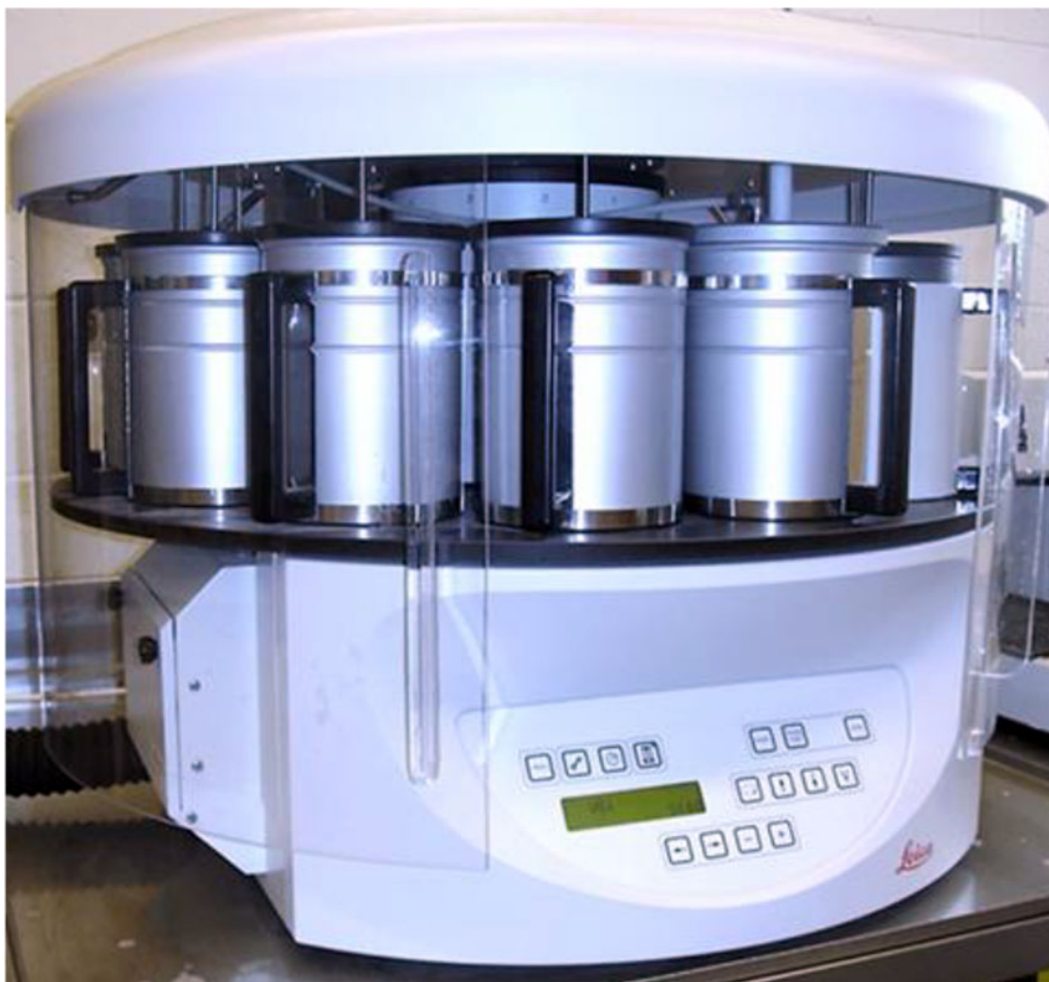
Figure 5. Leica TP1020 Automatic system for tissue histological processing.
